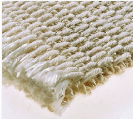
Solid woven carcass prior to PVC impregnation
