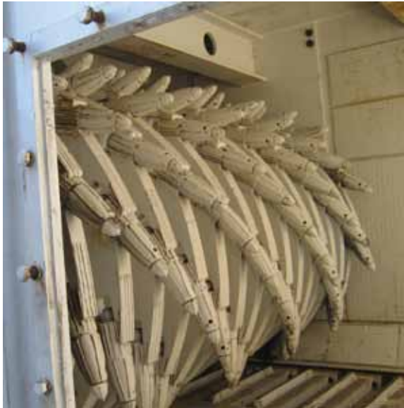
The carbide-tipped picks on the breaker shaft are designed to interlace with solid steel alloy flights to maintain a consistent minus 200 mm (8") product size.
