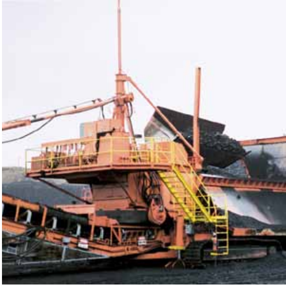
A mobile in-pit JOY Feeder-Breaker is used to size Powder River Basin coal to minus 8 inches at a throughput rate of 2500 Tons-per-hour.
