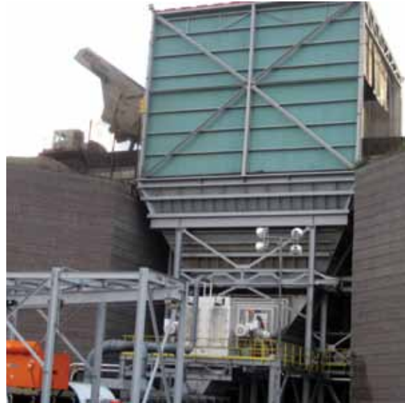
A stationary Feeder-Breaker receives coal and produces a minus 200 mm (8") product size at 6,000 TPH.
