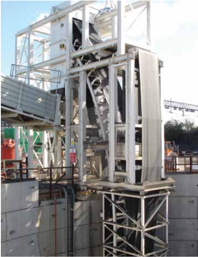
The HAC system is a proven method for conveying materials vertically from tunnelling operations to the surface.
