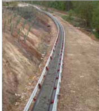
Shown above is a 1.87 km curved conveyor operating in the Scottish Borders, part of a 6 km system supplied to transport 1 Mt/y from an open pit mine to a lorry loading facility.
