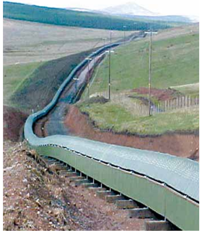
Shown above is a 1.87 km curved conveyor operating in the Scottish Borders, part of a 6 km system supplied to transport 1 Mt/y from an open pit mine to a lorry loading facility.
