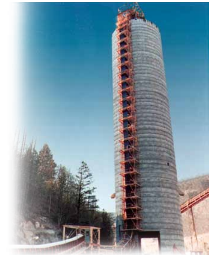
A 75 m vertical system lifting 750 t/hr of -127 mm size coal to the top of a rail car loading silo. Each of the 1,372 mm wide belts is powered by a 112 kw transmission.
