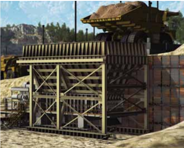
Skid mounted Feeder-Breaker breaking overburden to minus 12 inch product size at a variable rate of 0 to 5,000 TPH.
