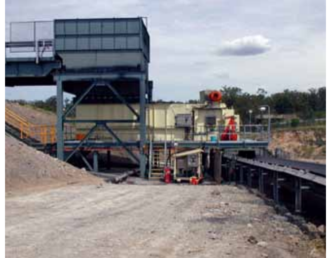
Stationary truck dump Feeder-Breaker running 1500 TPH of coal at minus 200 mm (8") output size.
