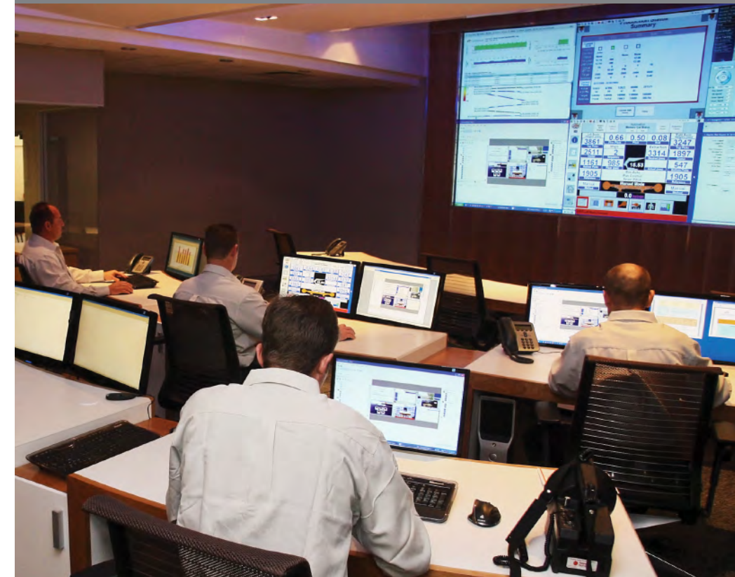
Health Management - State of the art predictive software analyzes the data streamed from your machines. The software predicts malfunctions, failures or process gaps at the earliest instance.
