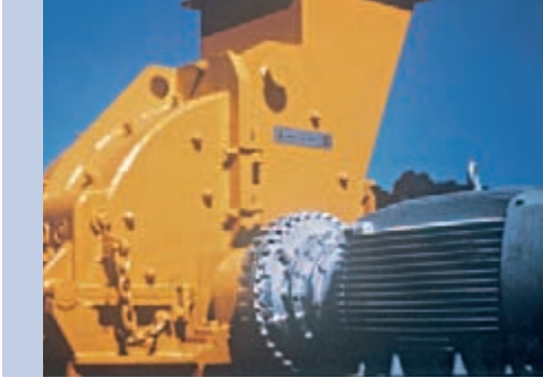
Optimum utilization of motor power using Voith fluid couplings on an impact crusher for reducing minerals.
